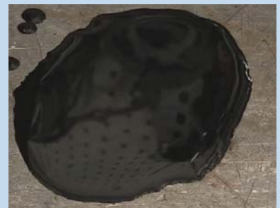
Transmission fluid should appear reddish and opaque like the fluid on the top. If ATF appears brown like the fluid on the bottom, it is past time to change it.
